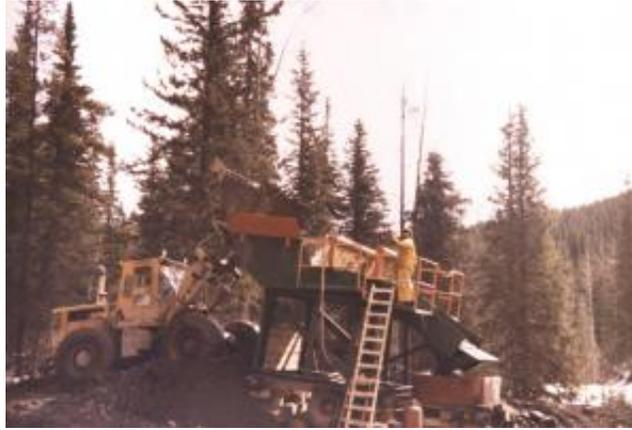
Frank had what was called a “grizzly” built at the logging camp which was the main tool he used in washing the gravel. He had built it so that there were no moving parts, just lots of jets spraying water down on the gravel the loader was dumping into the bin.
