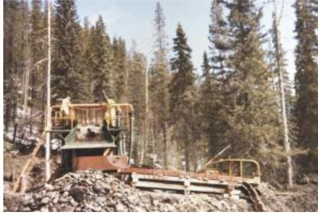
Once washed, the big boulders would roll down the front of the “grizzly” into a discard pile, and the gravel would drop down through the grates into the sluice.
