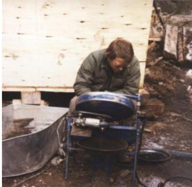
The gravel was then run through a spiral separating machine that would leave the gravel on the bottom and cause the gold to spiral to the middle and drop into a gold pan.
